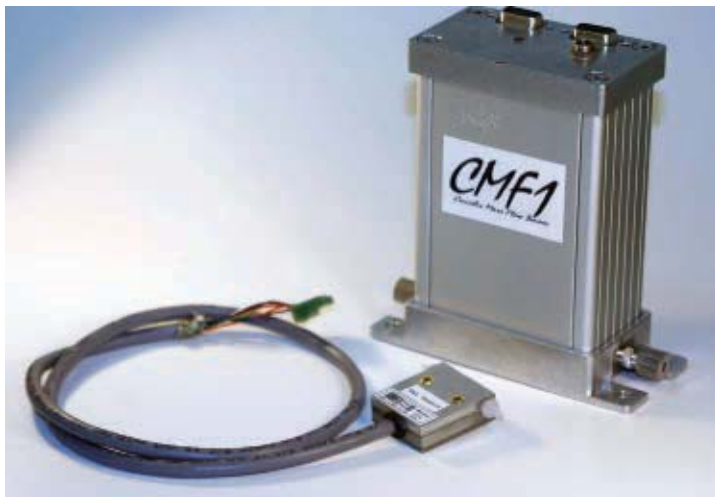
Figure 4. A Coriolis flow sensor typically used for direct methanol fuel cells in blended ethanol fuel applications.
