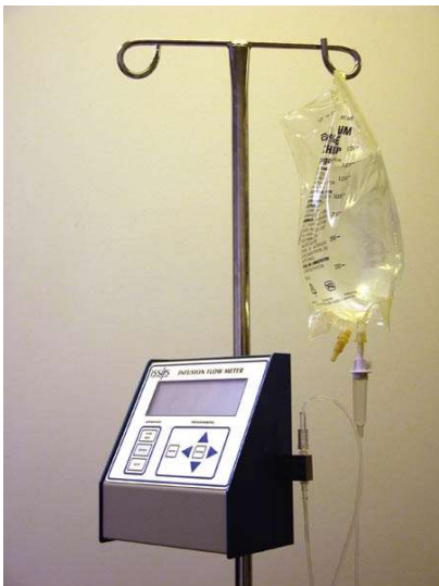
Fig. 5. A MEMS-based drug flow monitoring system.
