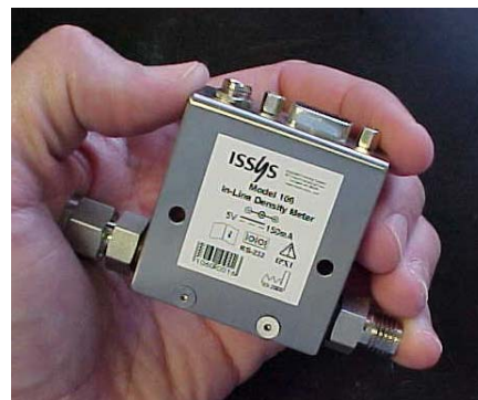
Fig. 8. A high flow rate by-pass, MEMS-based, resonant density meter.
